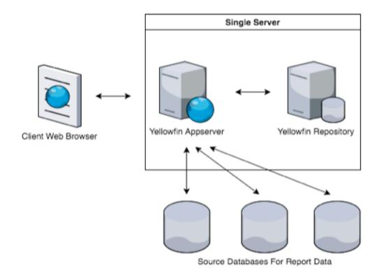
This is an ideal implementation for a small number of concurrent users. It minimizes hardware cost and installation effort to allow a rapid implementation of Yellowfin. This configuration removes any network latency between the Yellowfin application and the database server, but both systems share system
