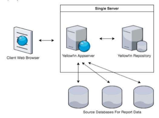
This is an ideal implementation for a small number of concurrent users. It minimizes hardware cost and installation effort to allow a rapid implementation of Yellowfin. This configuration removes any network latency between the Yellowfin application and the database server, but both systems share system resources.
