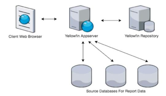
This configuration does introduce network latency between the Yellowfin application server and repository server, but does allow for an entire system to be dedicated to each component. Clustering from this configuration is also simple. Additional application server nodes can be connected to the repository for greater capacity.
