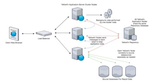
Each application server node added to the cluster increases capacity for supporting additional users. Processing load is distributed across available nodes.
